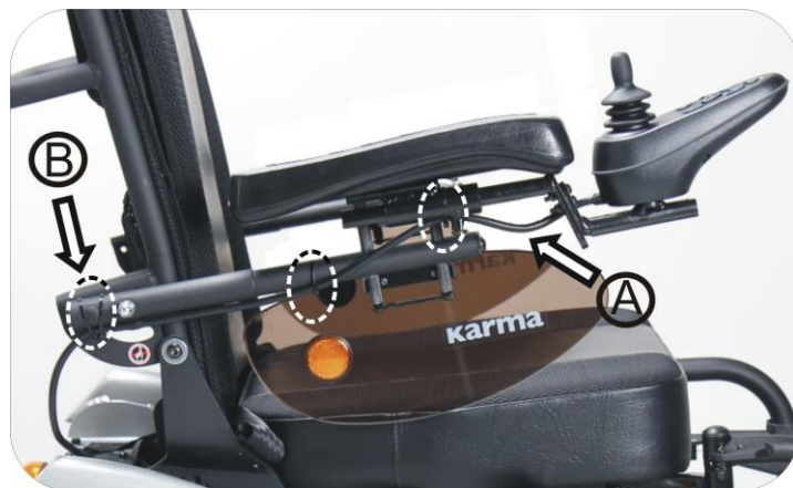
Controller Cable Tie Locations
